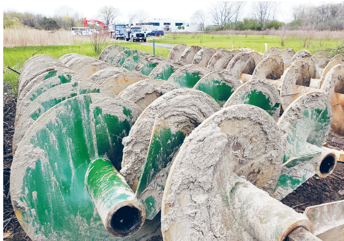
Eric Crump/H-F Chronicle Auger bits are lined up in preparation for horizontal boring through a section of Izaak Walton Nature Preserve.
